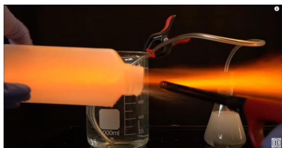
Figure 1. Burning of the hydrogen accumulated in a container.
