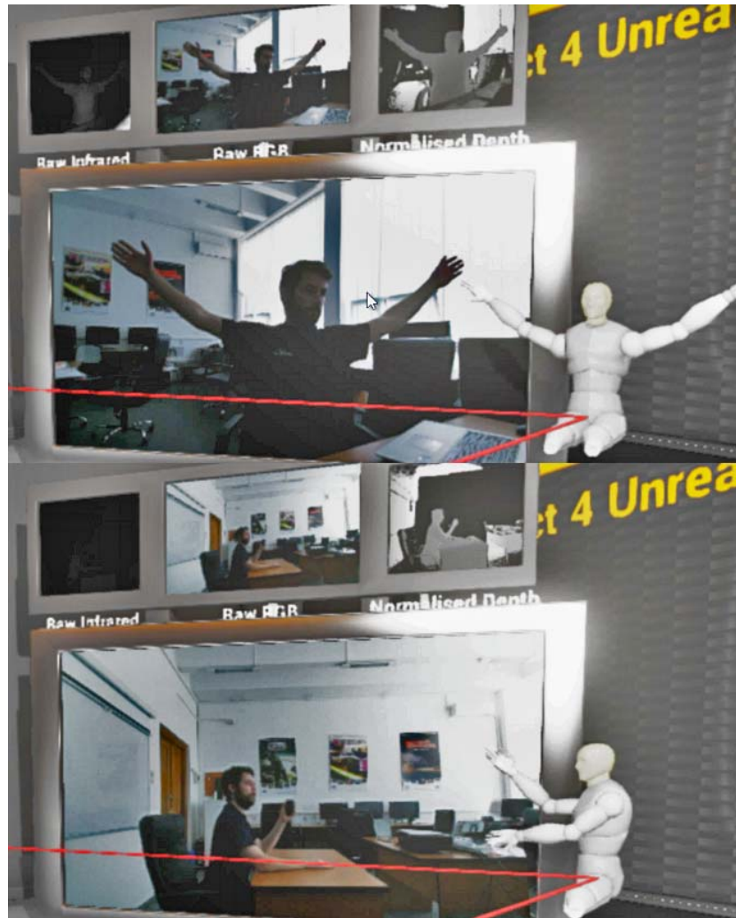
Figure 7. Kinect v2 accurate motion captures from different angles in a seated pose at a desk
