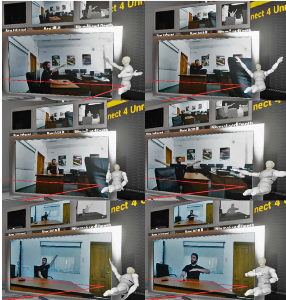
Figure 8. Kinect v2 motion capture in real-world home conditions (occlusion, reflective surfaces)
