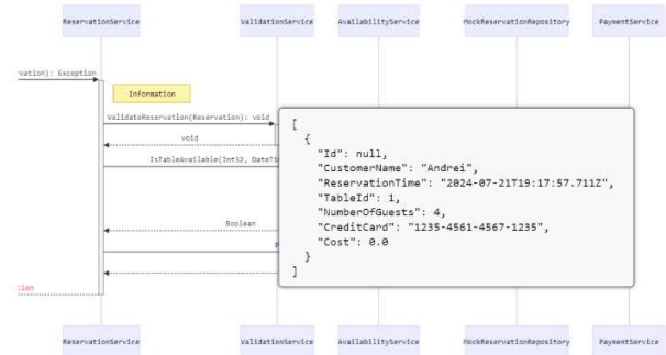
Figure 7. Displaying information about an exception that occurred in the execution of a scenario
