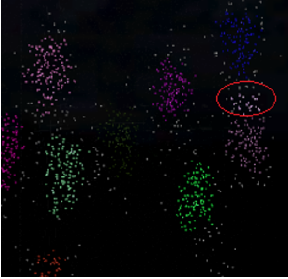
Figure 5. DBSCAN clustering on 3000 dataset. Over clustering highlighted by the red contour.
