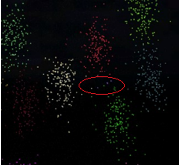
Figure 6. Mean Shift - Accurate clustering with minor outliers on 3000 dataset.
