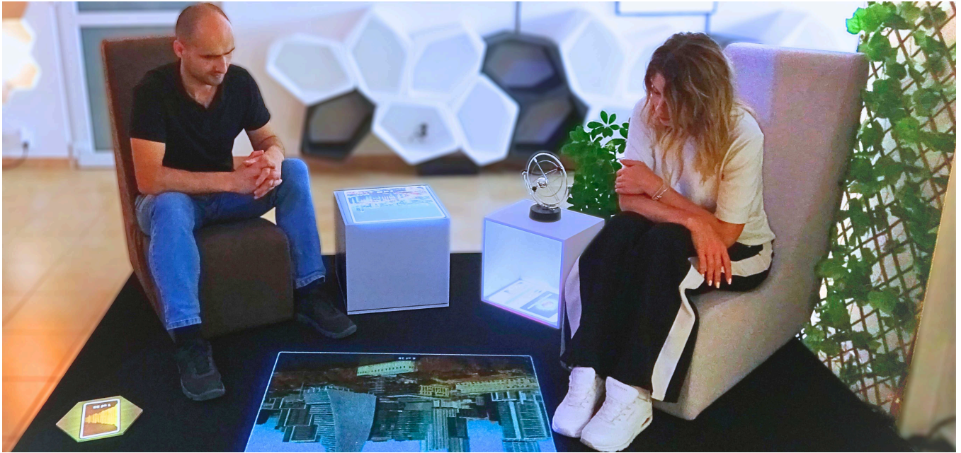
Figure 1: Example of a video-projected user interface enabled by our system for interacting with digital content displayed on different furniture surfaces, including the floor, a table, a shelf, and a polygonal surface in this photograph.
