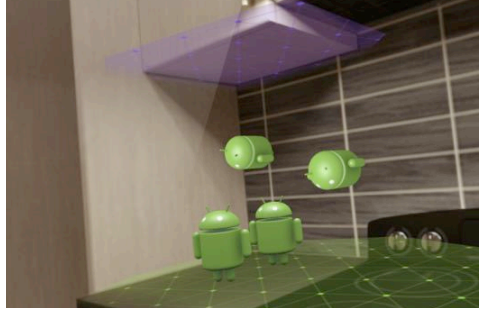
Figure 7. Real environment with virtual planar meshes and virtual objects – Unity (2019).
