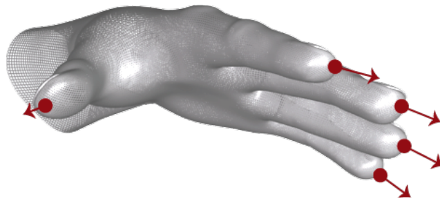
Figure 10- LeapMotion hand model: tip position and direction (Leap Motion Inc., 2018)
