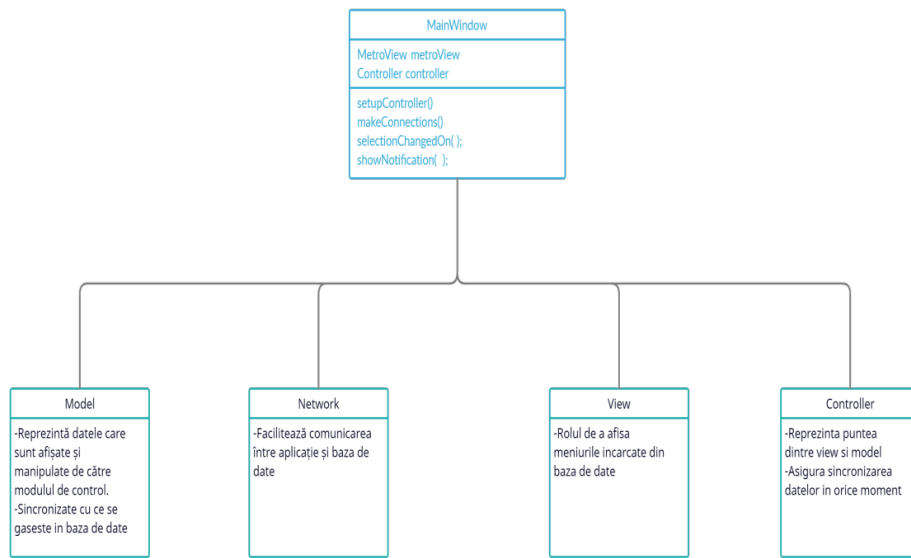
Figure 4. Main System Architecture
